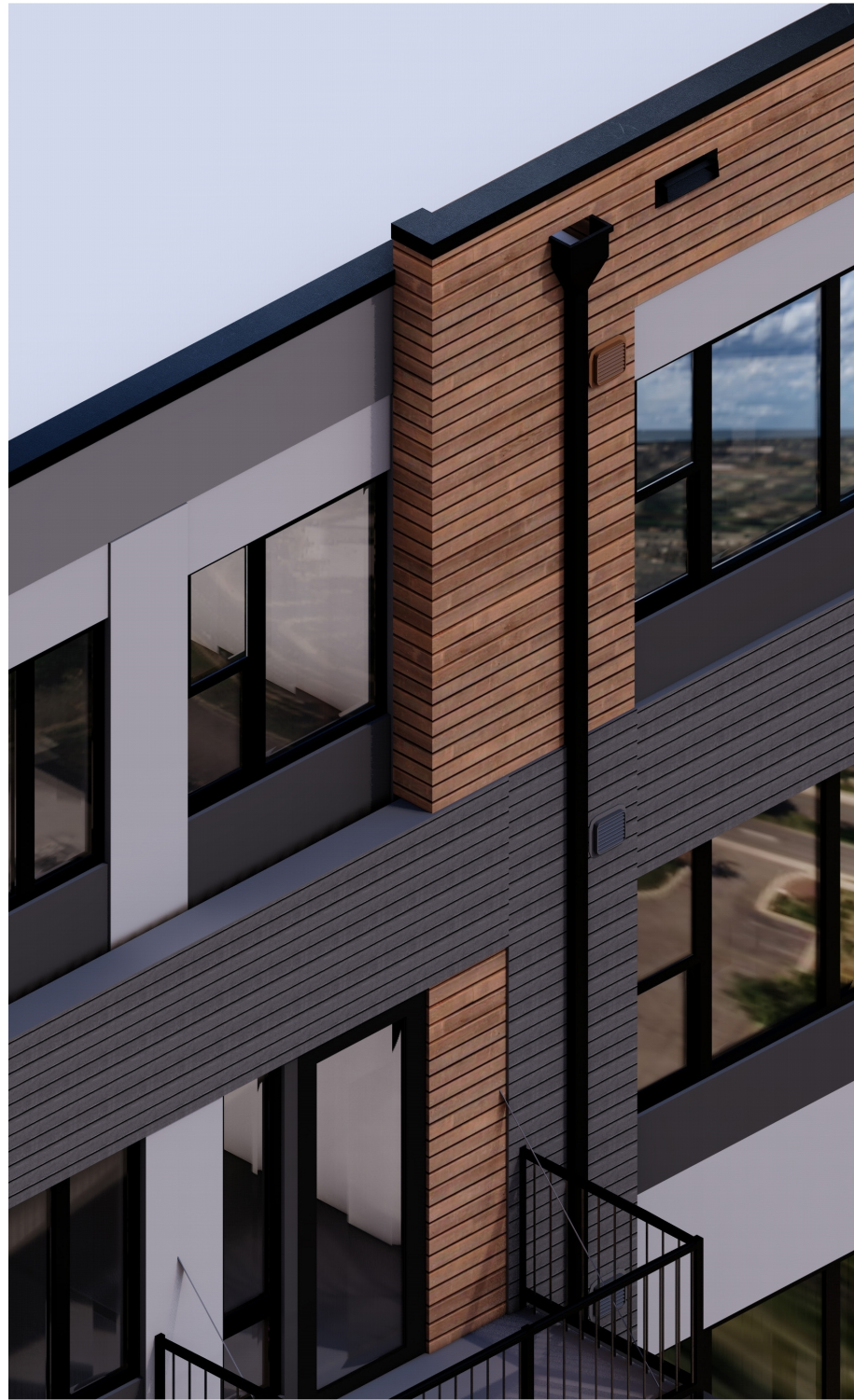
BLACK SCUPPER + DOWNSPOUT (6-8" RECTANGULAR DS)
