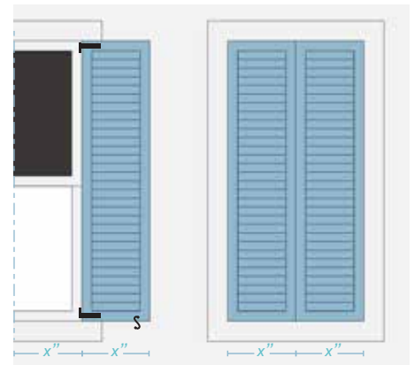
Shutters, fixed or operable, should align with the edge of the window frame, and be sized to cover half of the window opening. Shutter dogs hold shutters open against the wall.
