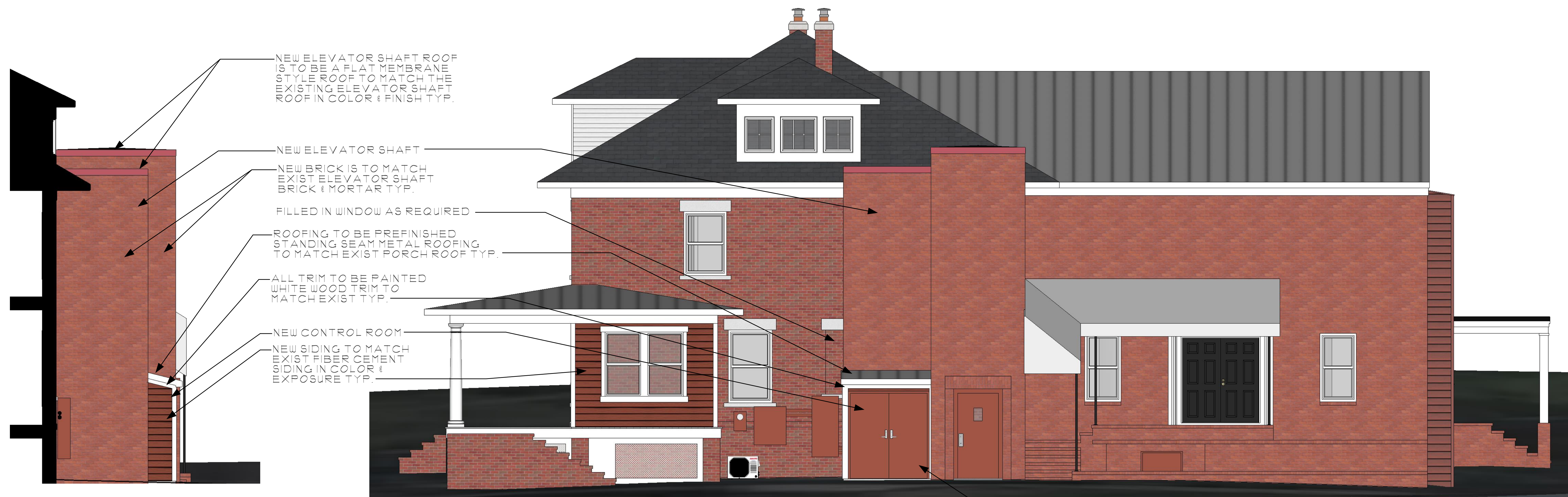
PROPOSED ELEVATOR NORTH ELEVATION 1/4" = 1'-0"
