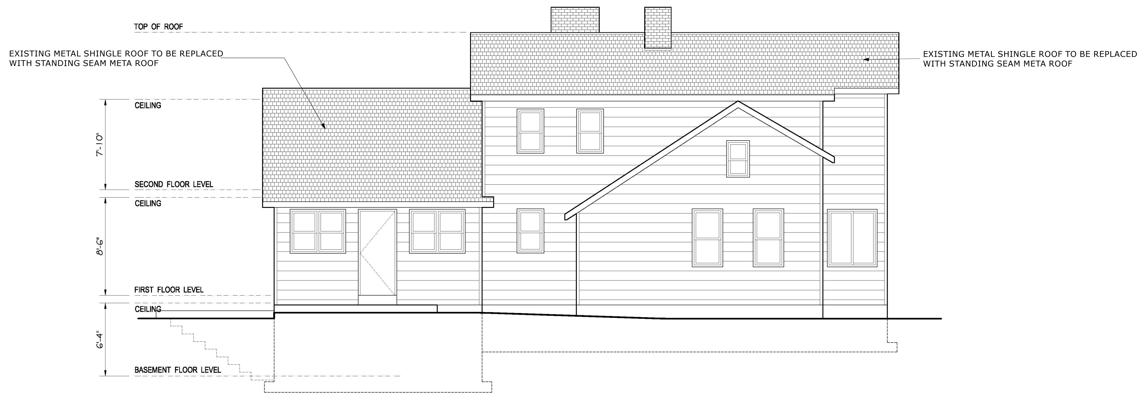
EXISTING REAR ELEVATION SCALE 1/4" = 1'-0"
