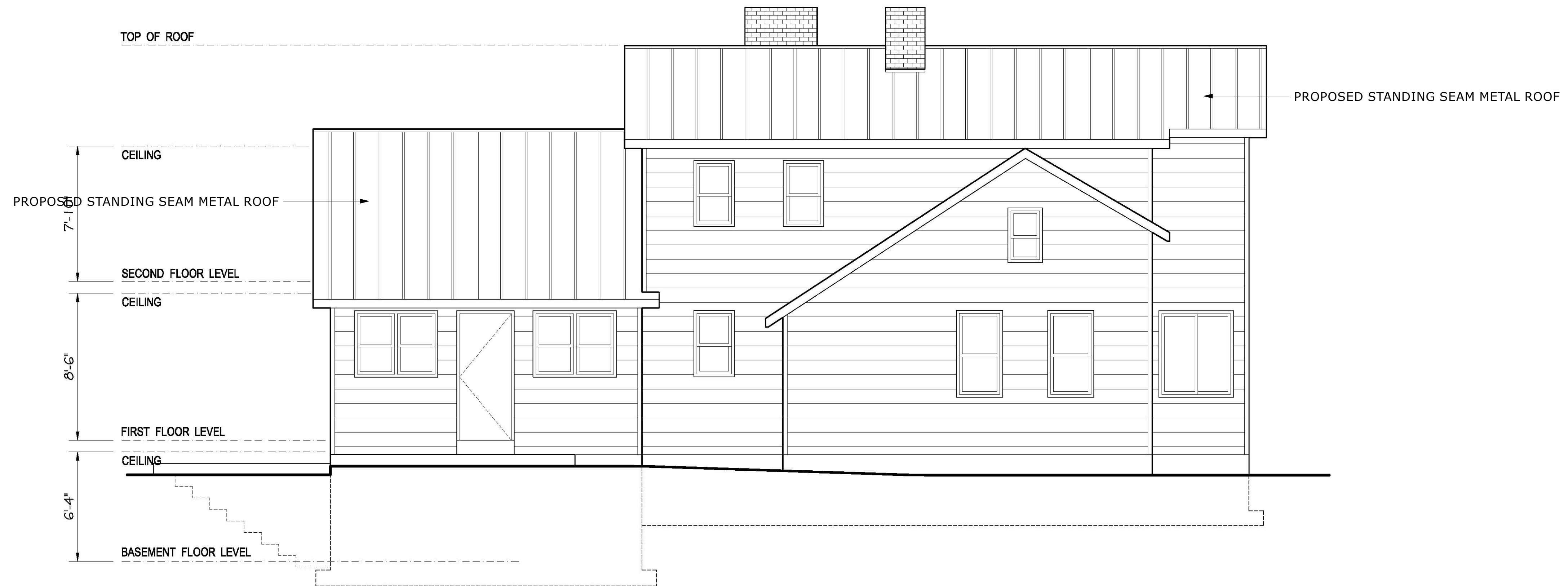
EX. / PROPOSED REAR ELEVATION (No Changes) SCALE 1/4" = 1'-0"
