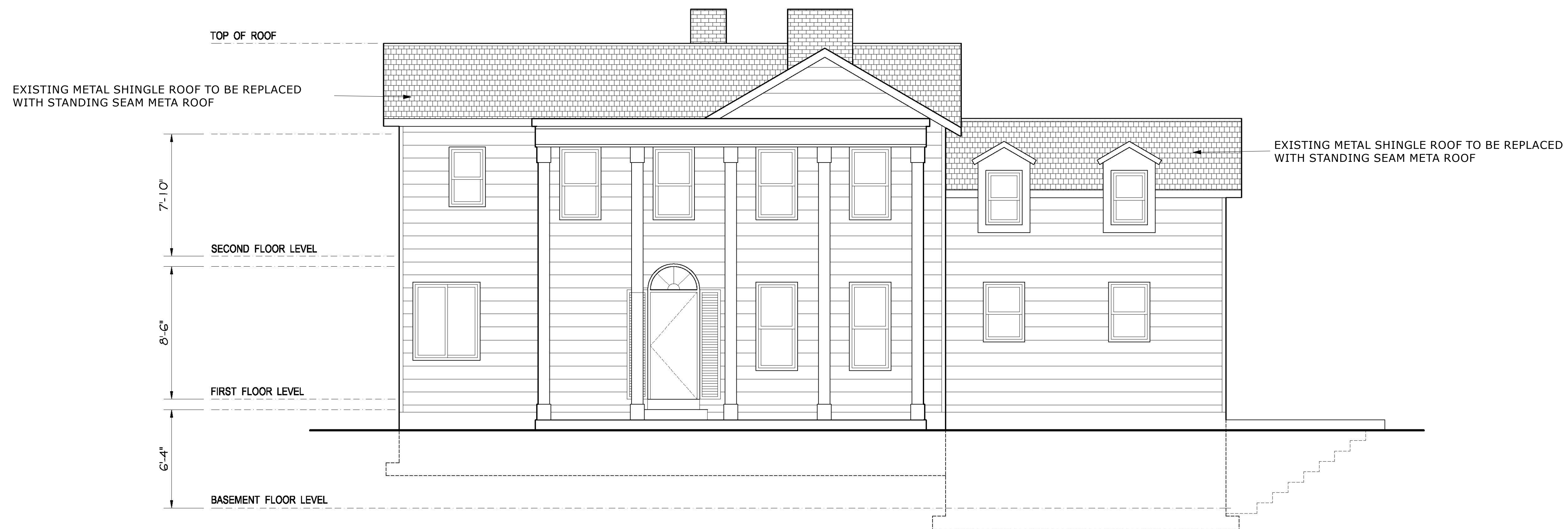
EXISTING FRONT ELEVATION SCALE 1/4" = 1'-0"
