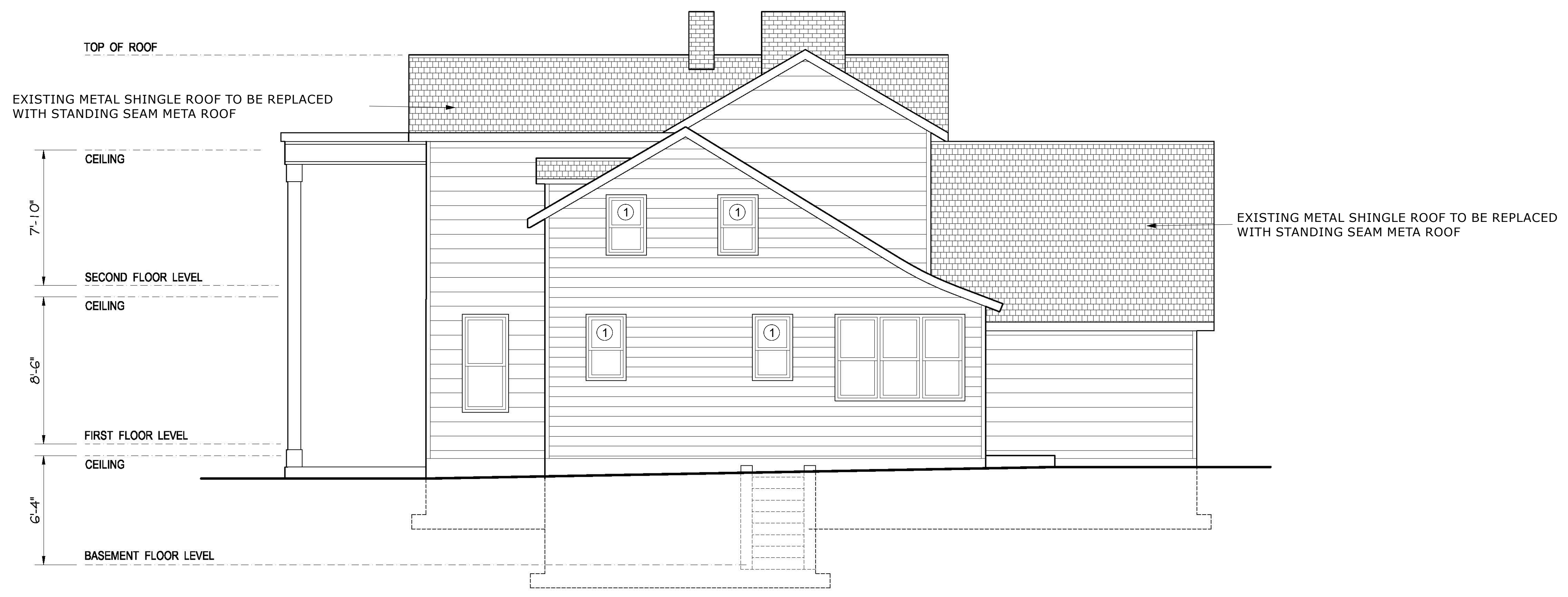
EXISTING RIGHT SIDE ELEVATION SCALE 1/4" = 1'-0"
