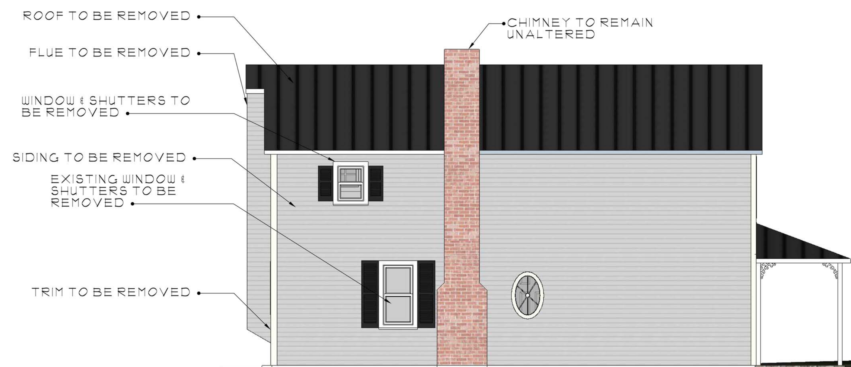
EXISTING LEFT ELEVATION
