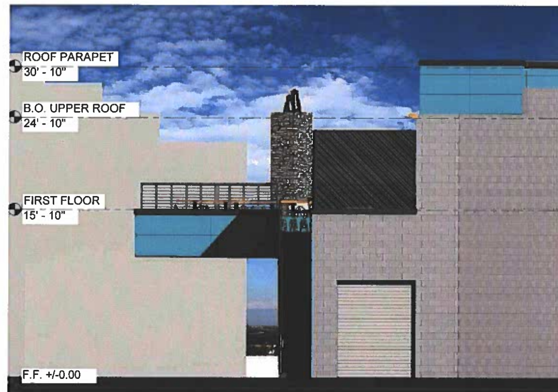
2 PROPOSED SOUTH ELEVATION 1/4" = 1' - 0"
