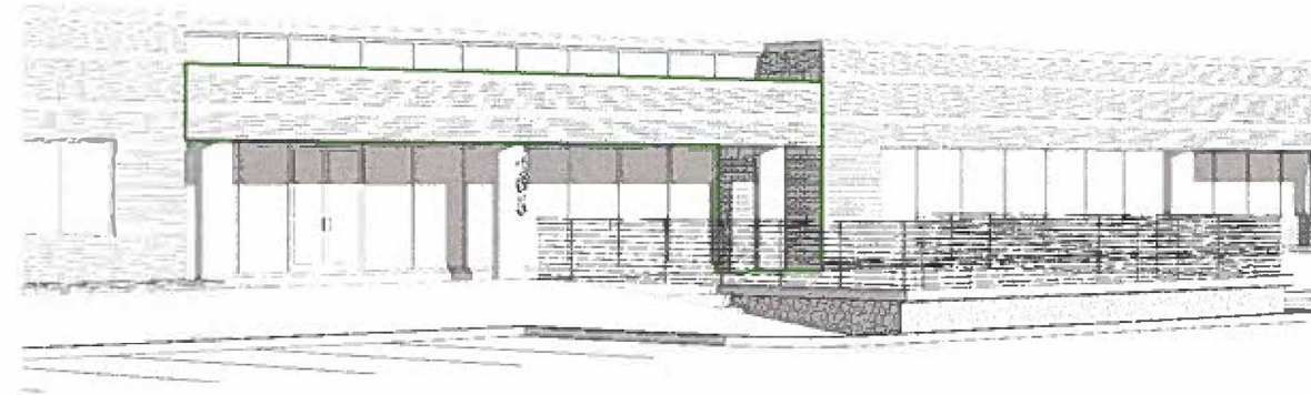
4 METAL GUARD RAIL C.R. LAURENCE CO., INC. ARS 200 SERIES SURFACE MOUNT CABLE RAILING, COLOR TBD
