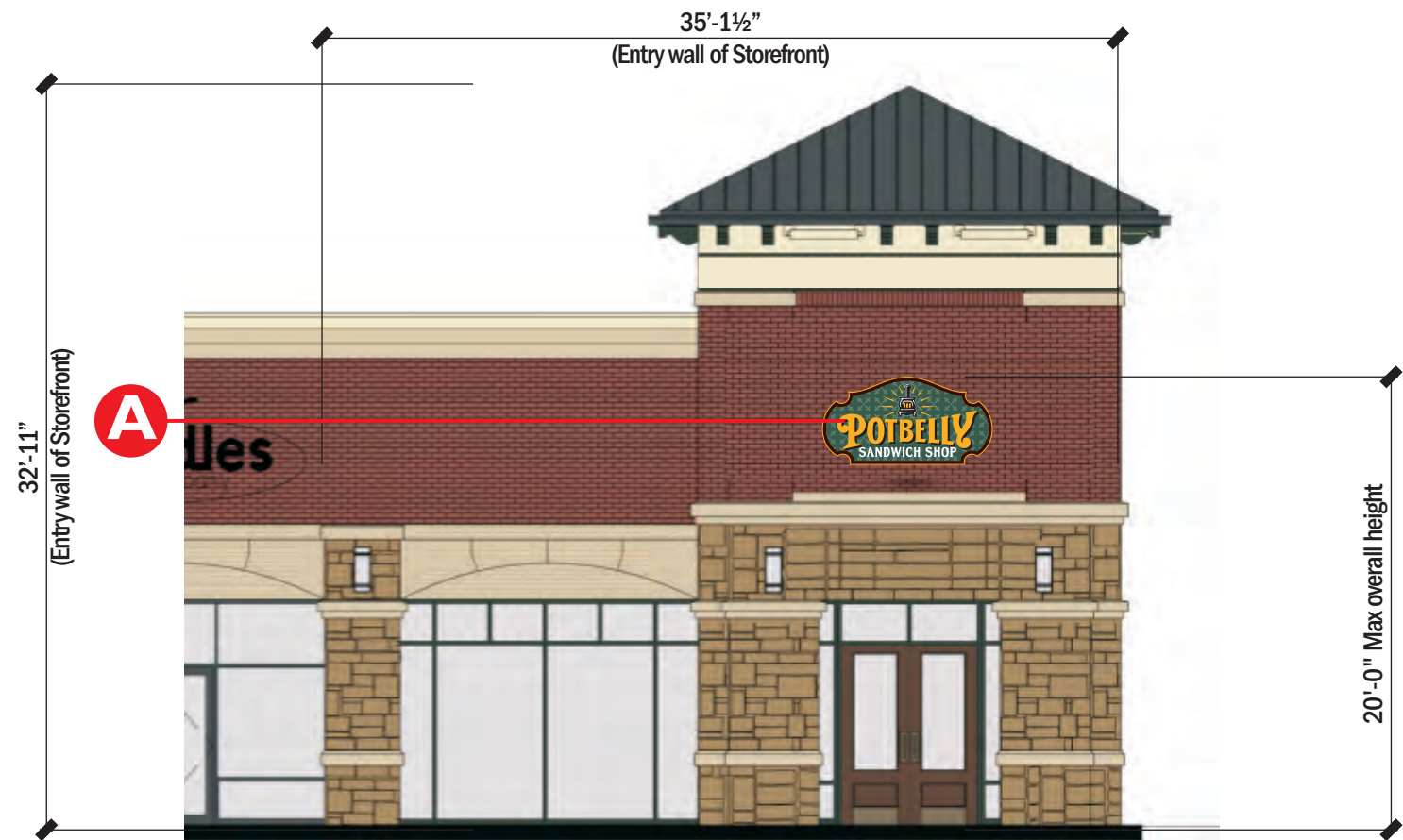
Building Elevation - North Scale: 1/8"=1'-0"
