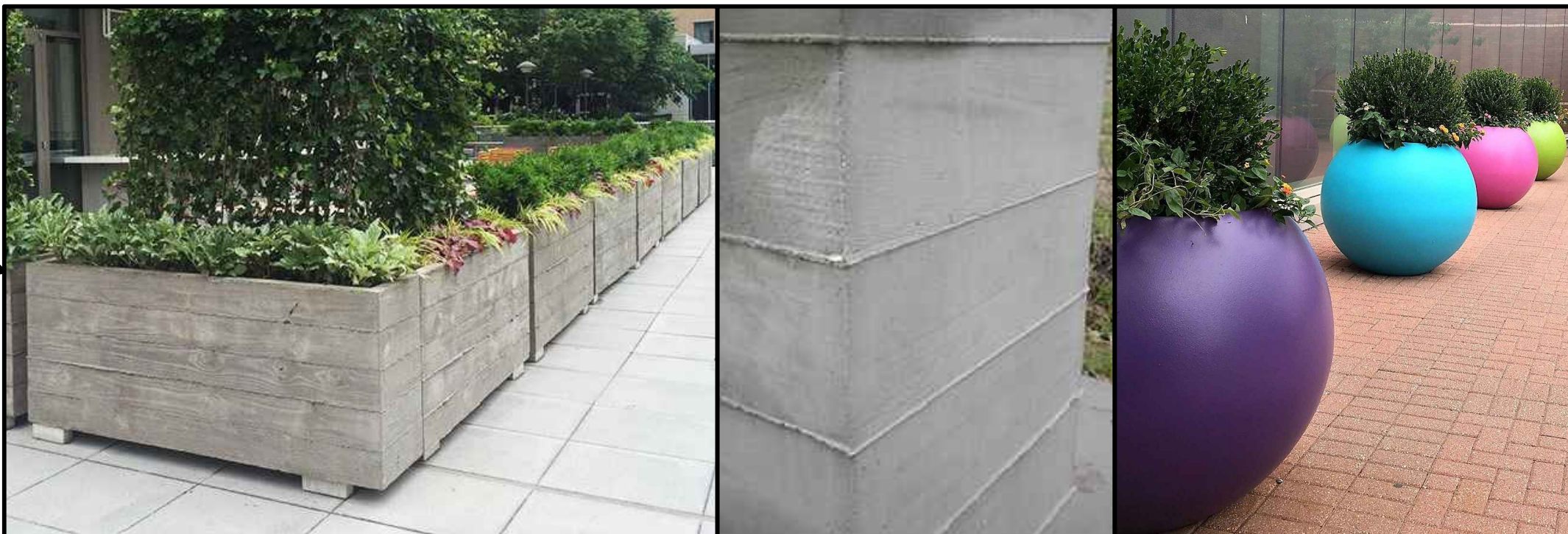
Planters - Wood grain concrete will match the seat/planter walls in the main section of the plaza. Texture matched wood used on architectural concepts and provides a "softer" and "casual" feel. Composite planters can accent entrances and bring color to facades around the remainder of the development in lieu of in-grade planters.
