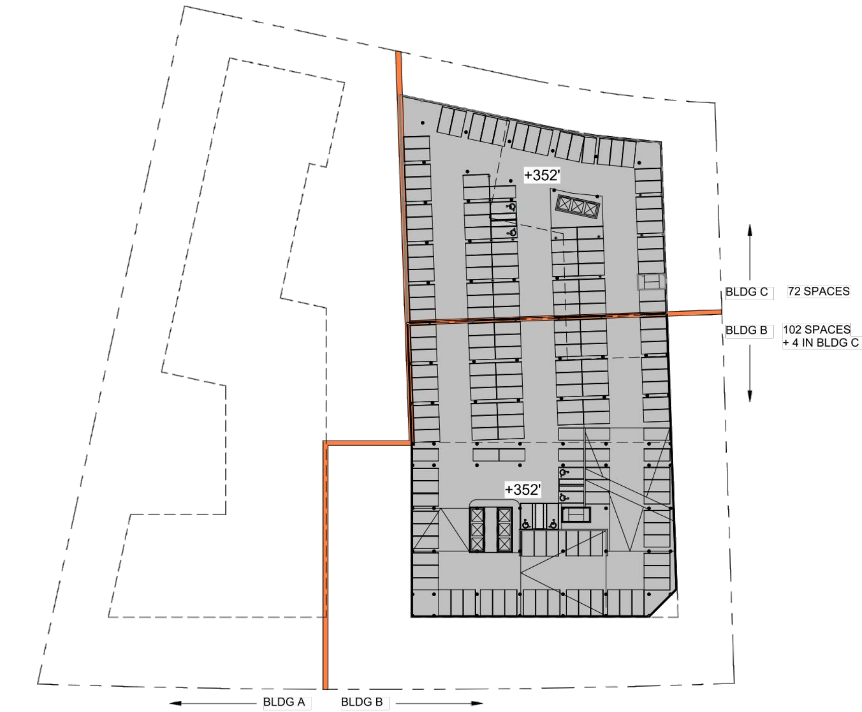
G2 LEVEL FLOOR PLAN SCALE: 1" = 60'-0"
