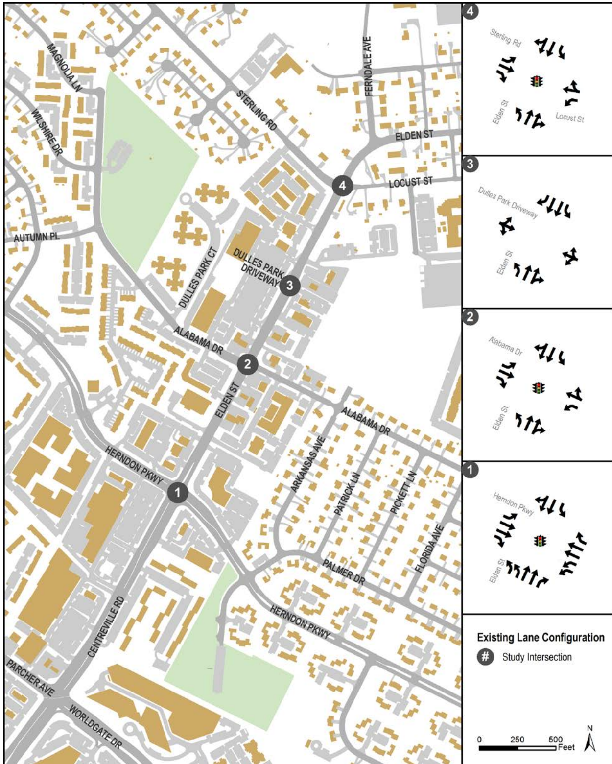
Figure 2 Existing Lane Configuration at Study Intersections
