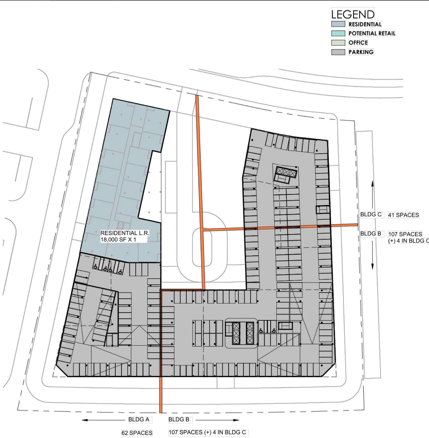
P3 LEVEL FLOOR PLAN SCALE: 1" = 60'-0"
