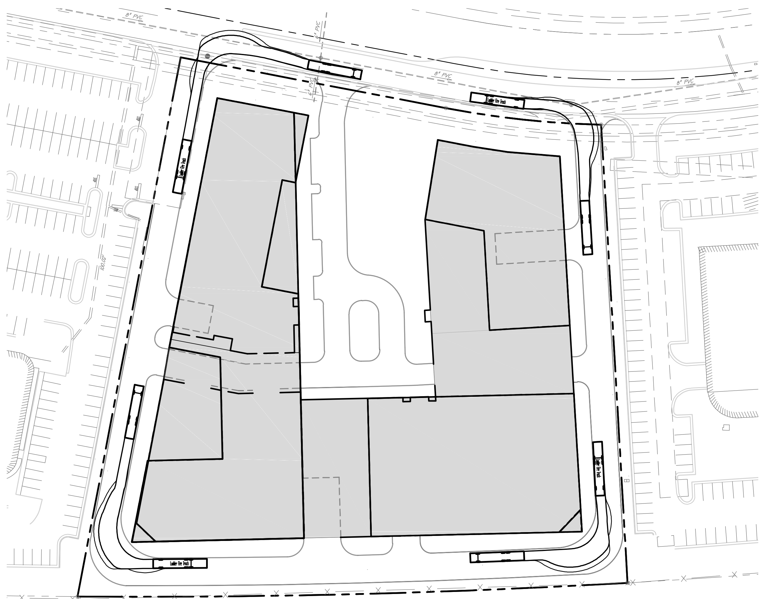
LADDER TRUCK TURNING: TURNING REAR OF SITE FROM SECONDARY ENTRANCE
