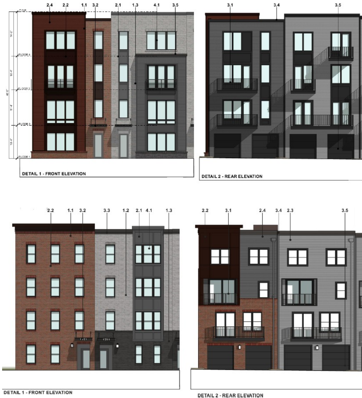
Figure 3: Front and rear elevations of stacked condos from the GDP (above); Proposed front and rear elevations of stacked condos (below).
