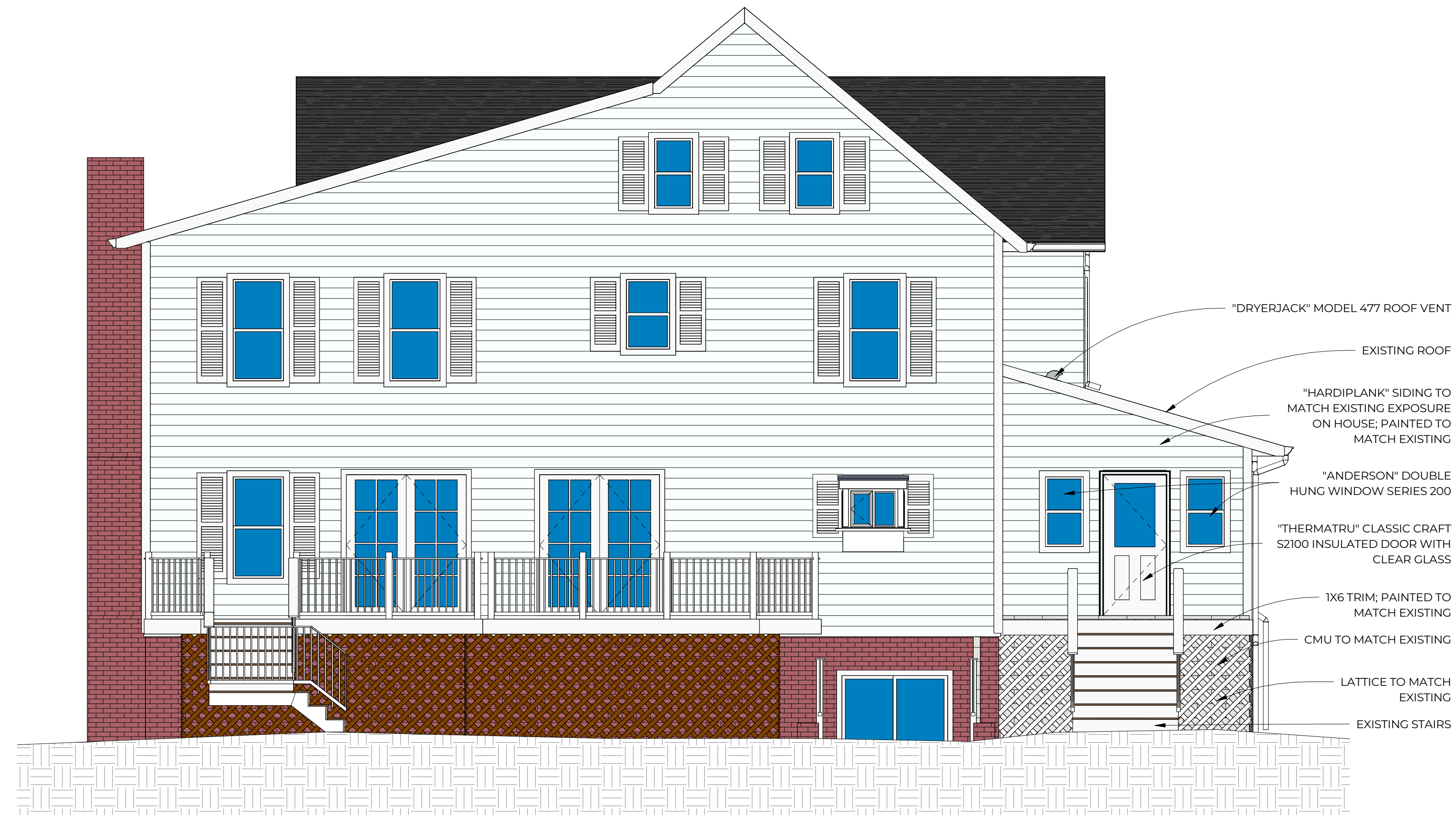
2 PROPOSED REAR ELEVATION 1/4" = 1'-0"
