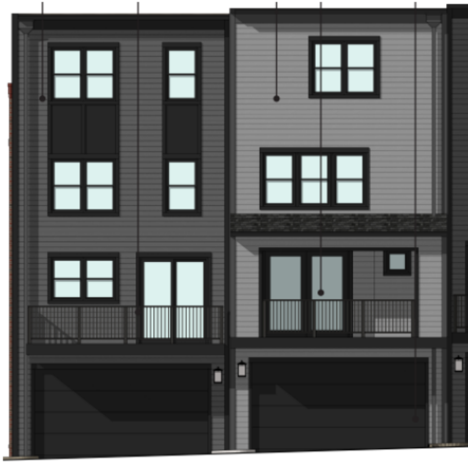
Figure 4: Rear elevation of the townhouse units showing the two available balcony types.
