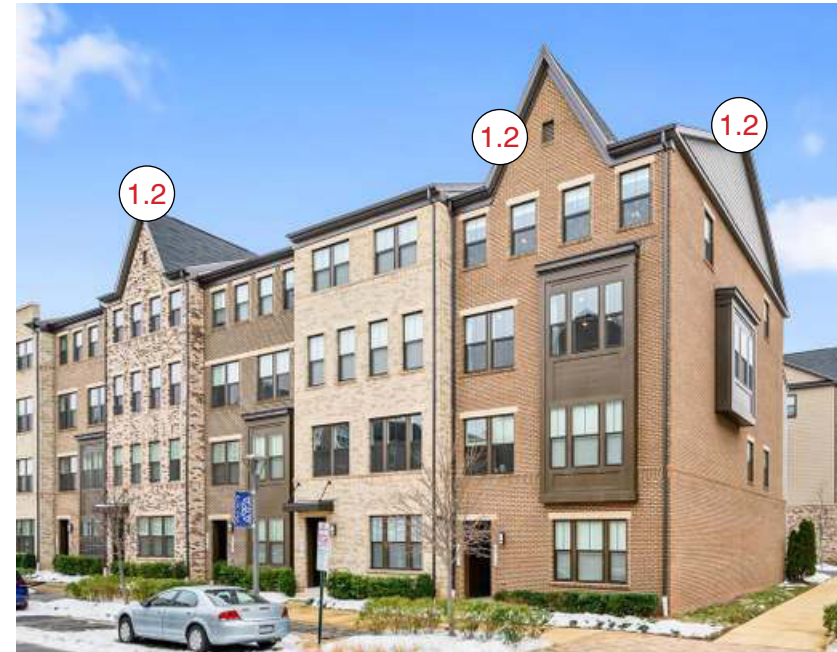
1.c SIDE FACING GABLE ROOF Includes front facing secondary gables identifying individual units
