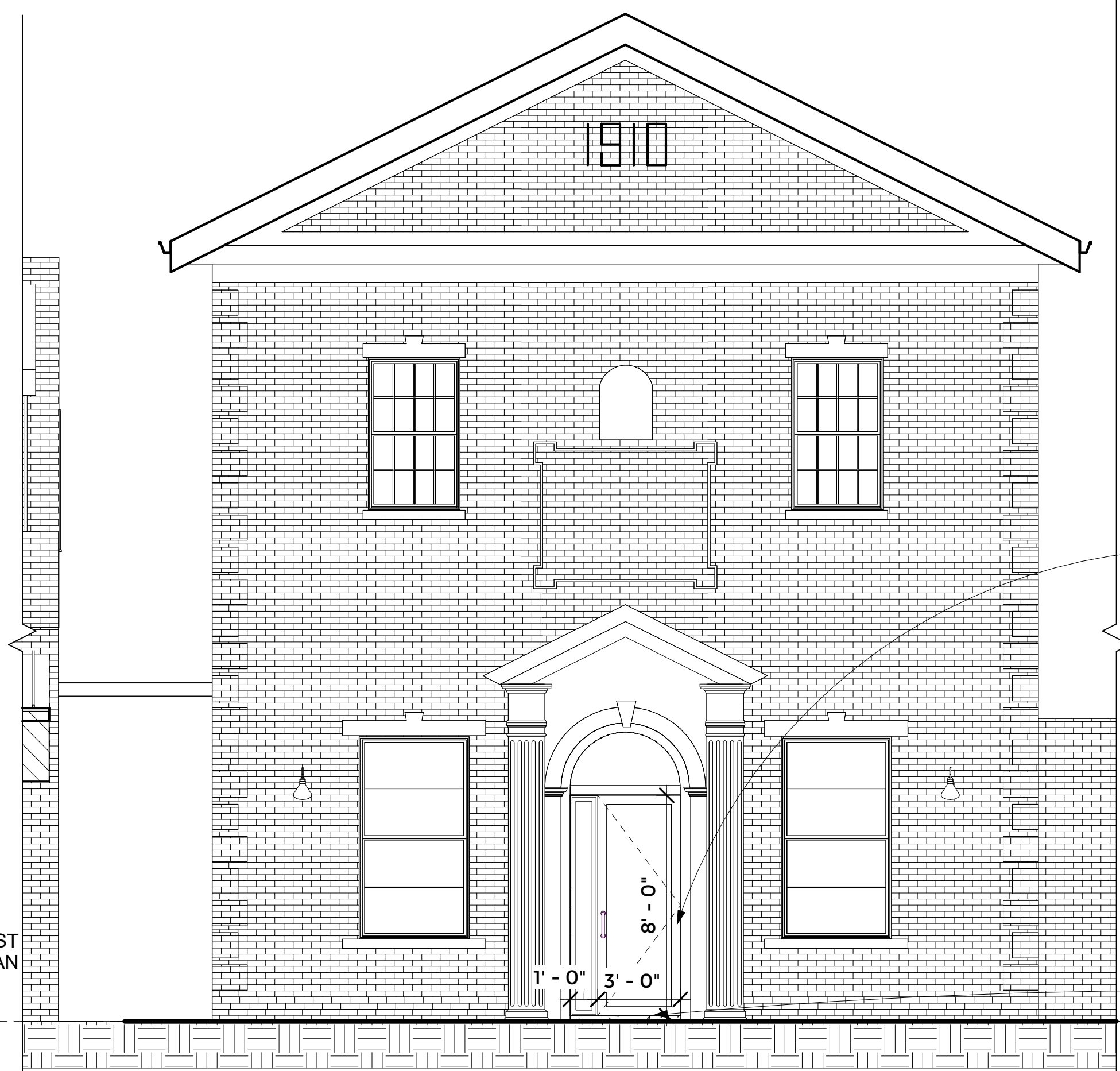
4 PROPOSED FRONT ELEVATION 1/4" = 1'-0"
