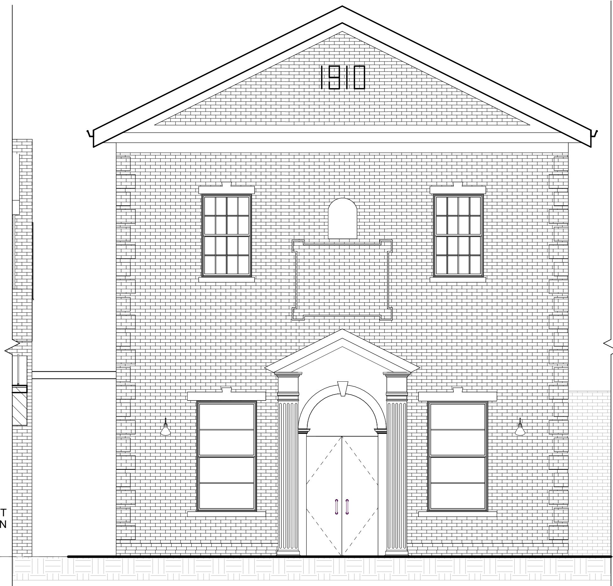
3 EXISTING FRONT ELEVATION 1/4" = 1'-0"
