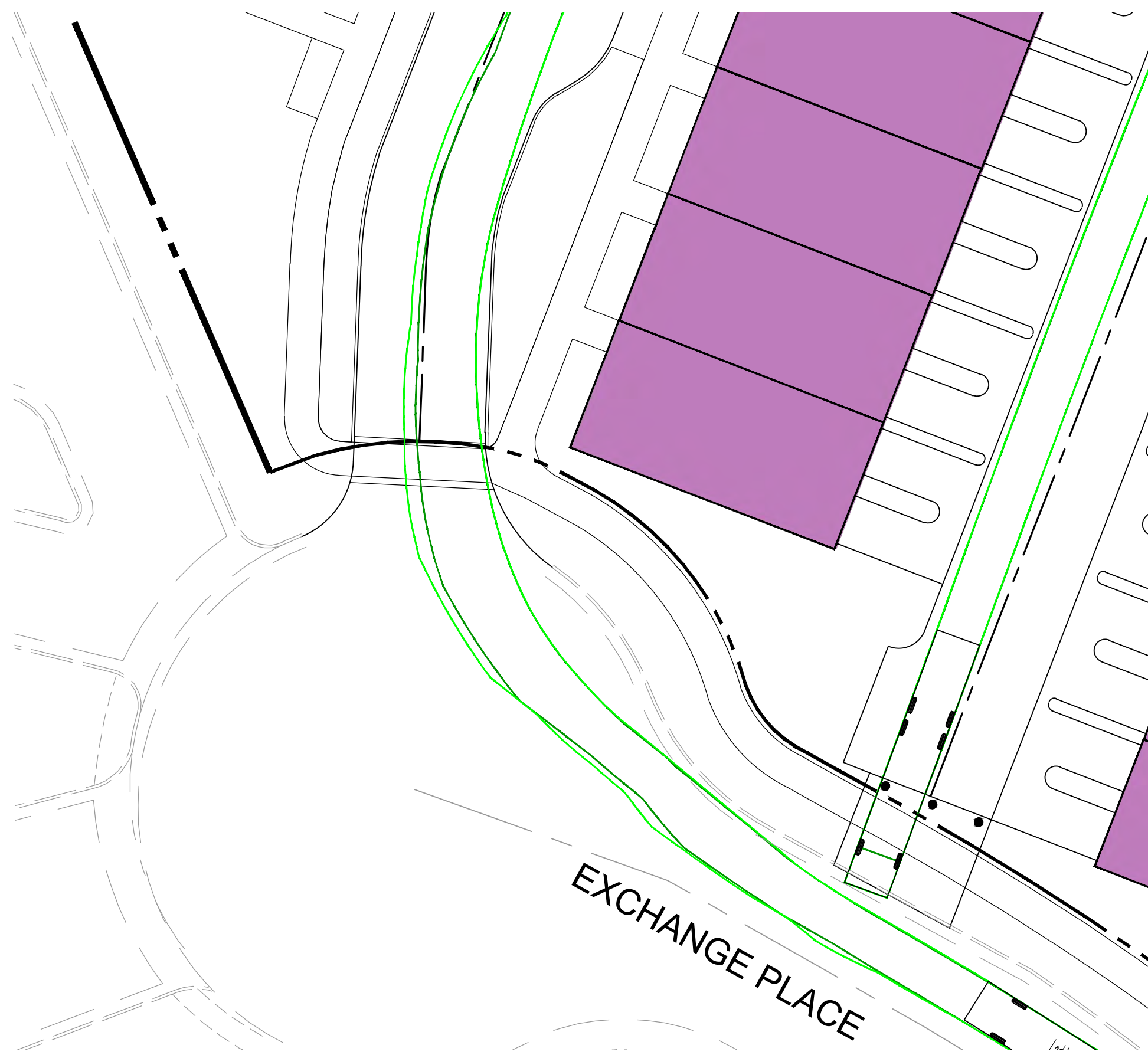
FIRE APPARATUS ENTERING TOWNHOME ALLEYWAYS FROM EXCHANGE PLACE
