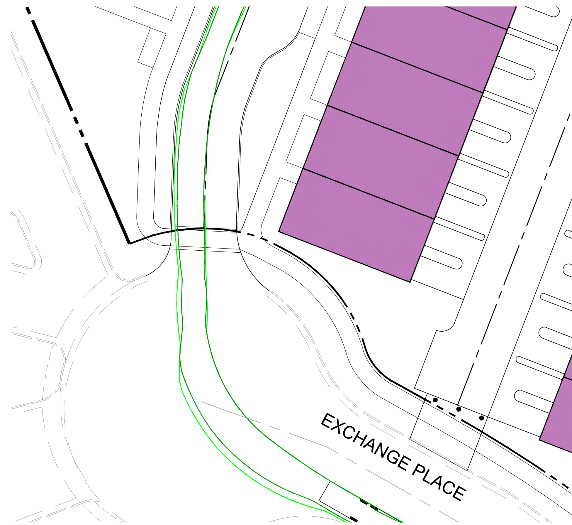
FIRE APPARATUS EXITING LEFT TURN TO EXCHANGE PLACE
